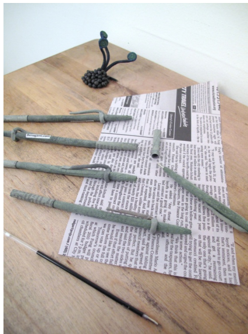
The new material was developed for use in his Origami Bonsai sculpture. “Green” paper pens are made by rolling newsprint around a ball-point pen refill.
